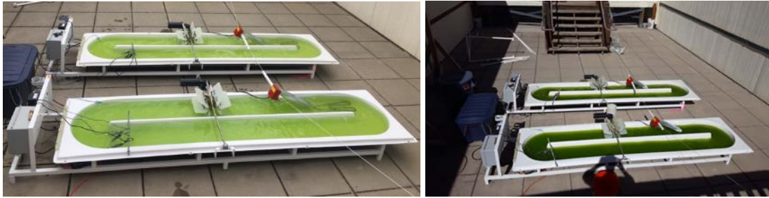
Figure 25. Cultivation of alga consortia that contains strains PW-95, WC-1, and X. Each respective culture was grown individually in the laboratory and then combined into a single inoculum. The consortia were grown outdoors for two weeks in 200L (~53 gallon) raceway ponds. A paddle wheel insured mixing and a modified livestock trough heater maintained a water temperature >15 °C.
