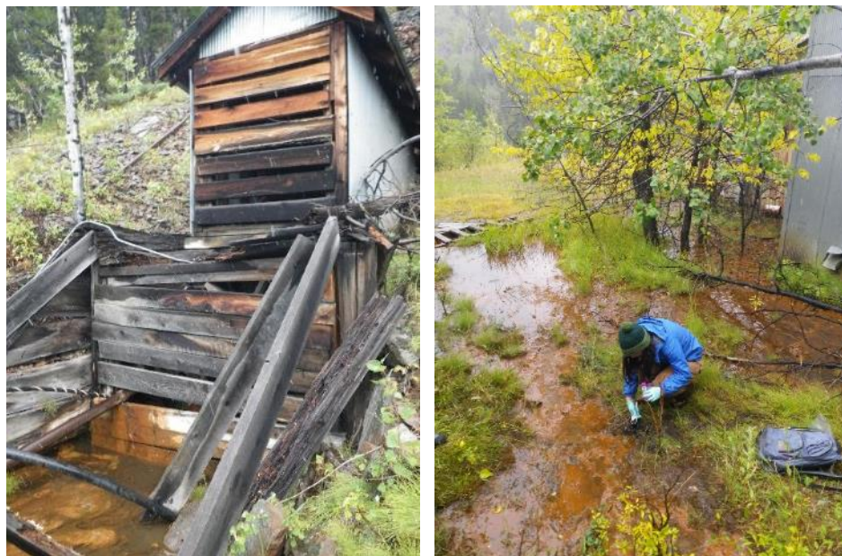
Figure 9. Left: Mine adit with water flowing out of shaft at Evening Star in Carpenter-Snow Creek Mining District. Right: Graduate student Emily Stoick sampling sediments from the adit discharge area at Evening Star to cultivate native bacteria capable of metals remediation.
