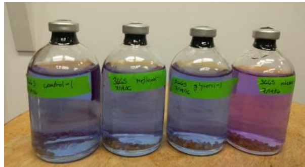
Figure 12. Left: Deployment of microbial sampling chambers into wells at Colstrip. The chambers contained sand for attachment of bacteria present in the aquifer. Right: Set of batch bottles with sand as inoculum for growth and selenium removal studies. Pink indicates microbial activity has depleted the oxygen in the bottle.
