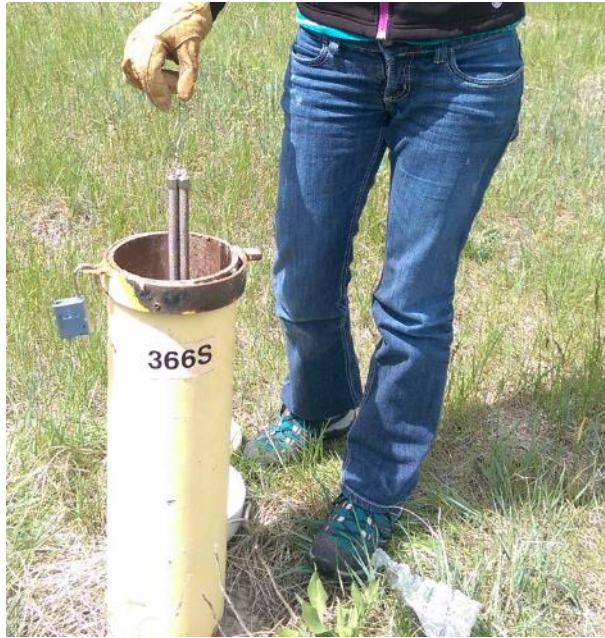
Figure 12. Left: Deployment of microbial sampling chambers into wells at Colstrip. The chambers contained sand for attachment of bacteria present in the aquifer. Right: Set of batch bottles with sand as inoculum for growth and selenium removal studies. Pink indicates microbial activity has depleted the oxygen in the bottle.
