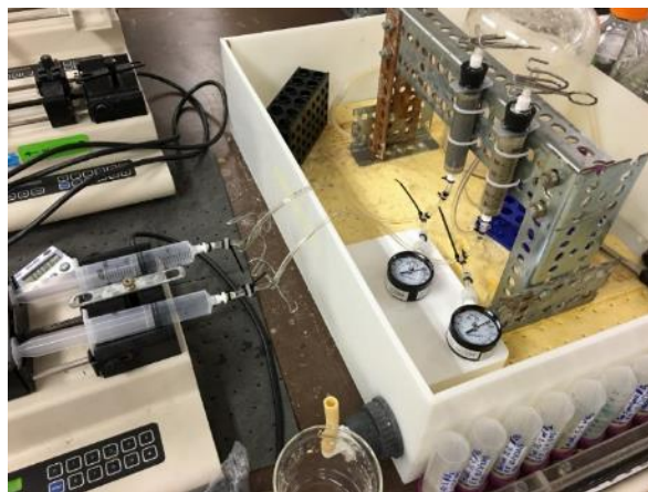
Figure 5. Experimental column set up. A syringe pump was used to inject MICP promoting solutions into a column loaded with sand and fly ash (column of the right). Permeability of the fly ash/sand mixture was observed to decrease over the course of the 20 injections of MICP promoting solutions.
