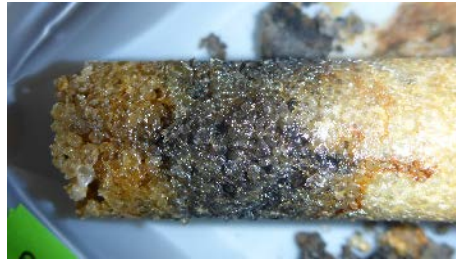
Figure 3. Thermally induced calcium carbonate precipitation cemented together particles of sand after removal from the steel pipe batch reactor.
